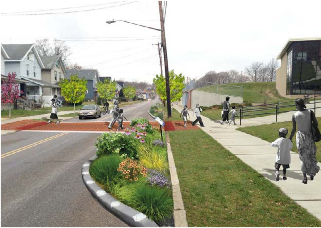
Rendering of the proposed crosswalk and vegetated curb extensions along 5th Avenue in front of the Robinson School. The openings in the curbs allow stormwater to enter the vegetated curb extensions, sustaining the native plants. Interpretive signage placed within the plantings inform the students on the project's ecological benefits.
